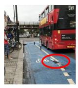
8. Ritherdon Road junction. A near miss between a van turning left into Ritherdon Road and a P2W continuing ahead was observed during the site visit. This may indicate that the reliance on the No Left Turn signs on the traffic signals may not be sufficient or that enforcement is required (note that this was observed before the commissioning of the bus gate was completed).
